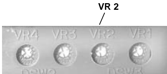
POTENTIOMETERS ARE LOCATED UNDERNEATH A FLIP - DOWN COVER OF THE FRONT PANEL
